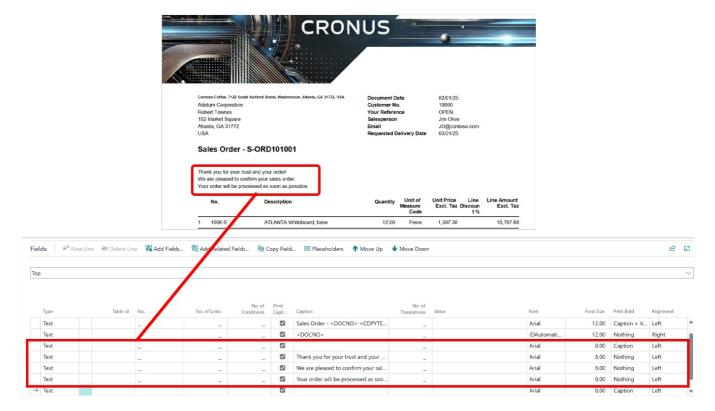
You have added a line of text to a layout area. You can move the individual text lines by proceeding as described in the section Move Field in Report. Placeholders can be used in these text lines to place report-specific field values in the text lines. Further information on placeholders and their use can be found in the section Add Placeholder to Text Line.
